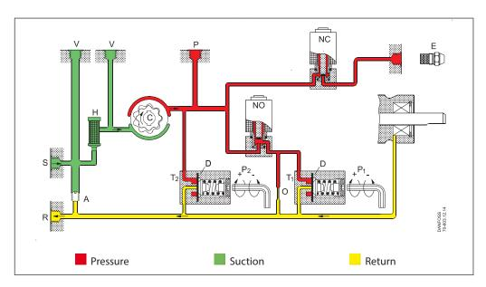
From the suction inlet (S) fuel is drawn through the filter (H) to the gear set, where the pressure is increased. By means of the diaphragm (D) in the pressure regulator for stage 1 ( $T_1$ ), the pressure is kept constant at the value set on adjustment screw ( $P_1$ ).
