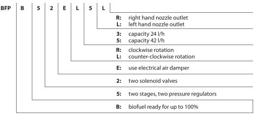
Nozzle capacity at 4.3 cSt., 10 bar, 2800 min<sup>-1</sup>
